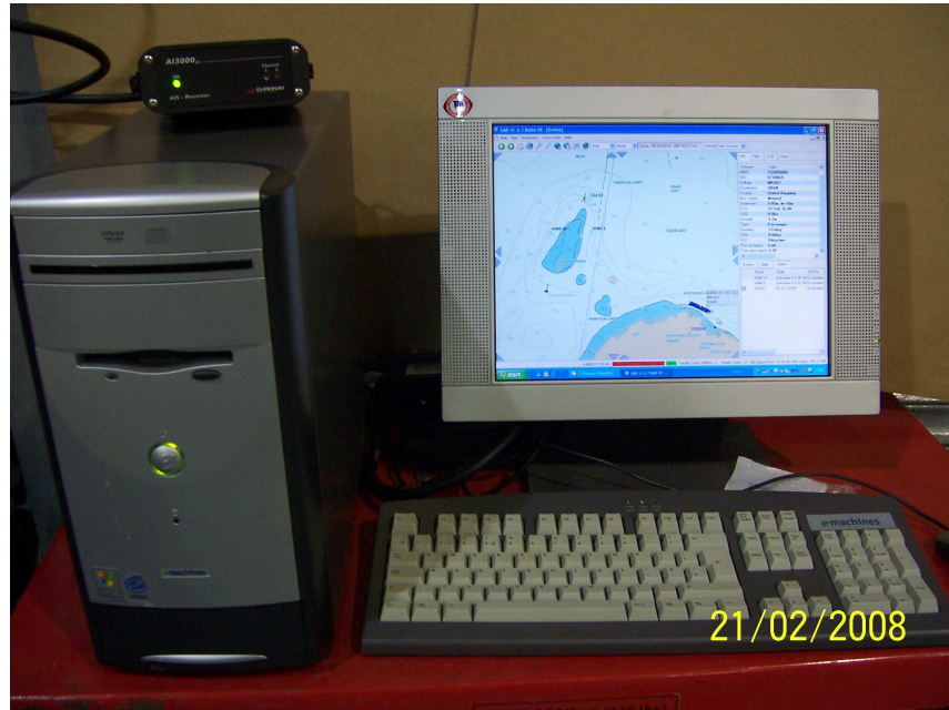
Figure 5: ECS equipment set up, showing the AIS unit, ECS PC and display.
